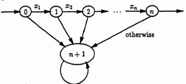
where 0 is the initial state, n is the accepting state and n+1 is the fault state.
