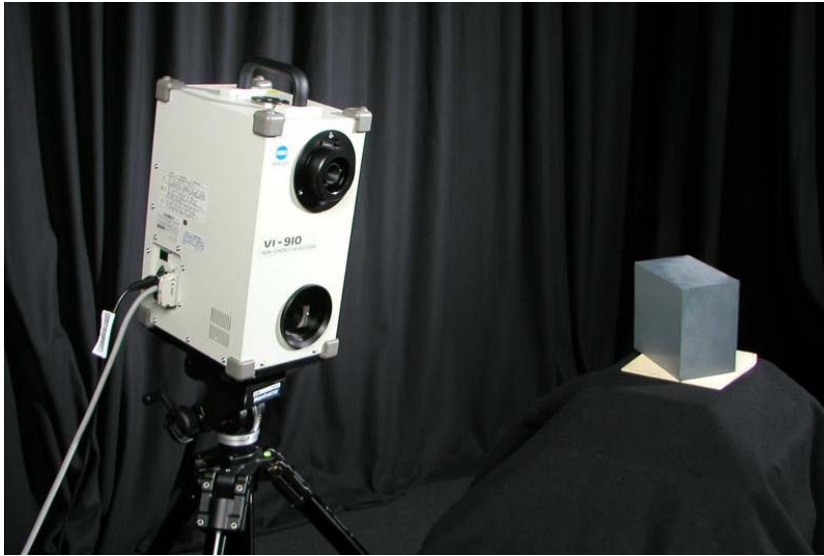
Figure 4.1: The setup used for test scans consisting of a Minolta VI-910 laser range scanner and the 90° calibration target.
