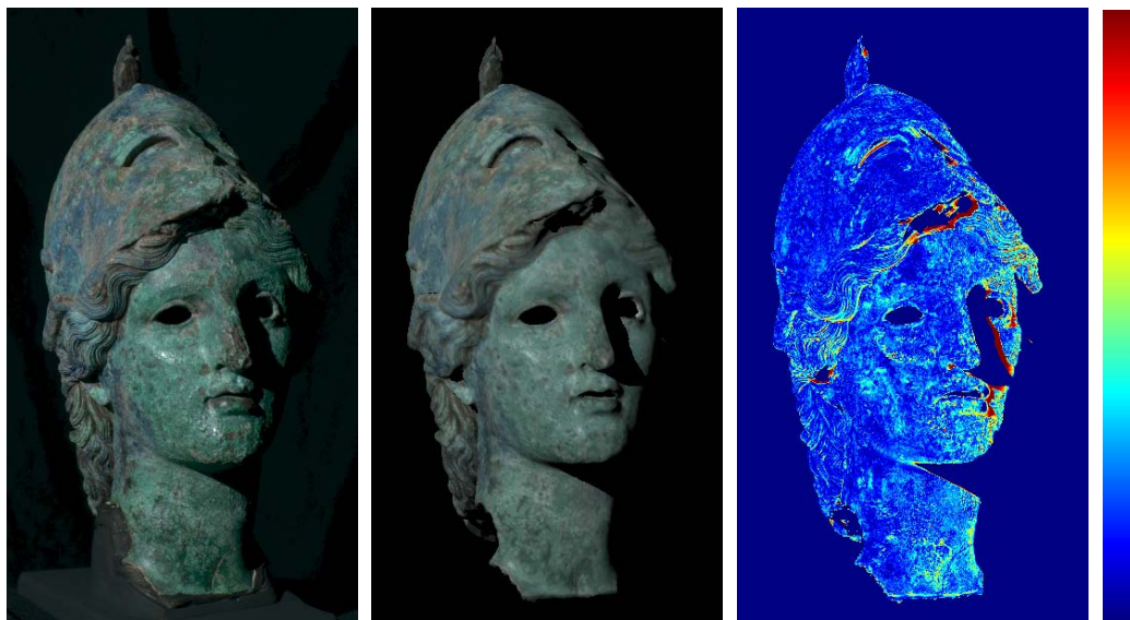
Figure 5.3: From left to right: Photograph of the corroded bust, rendered BRDF model, and difference image ( \Delta E ). The false-color difference image covers the range of [0, 50] ; areas with larger difference (mostly misaligned shadow boundaries) were cropped.
