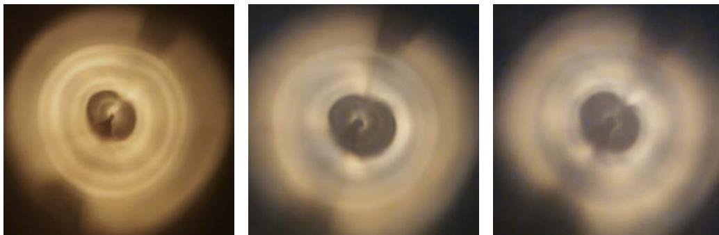
Figure 6.16: Left: Photograph of the flashlight illuminating a plane at 75 cm distance. Middle: Reconstruction of the same setup from data measured with a filter of 30 mm width. Right: Reconstruction from data measured with a filter of 20 mm width.
