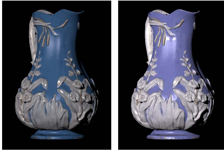
Figure 5.1: Calibrated (left) and uncalibrated (right) carafe dataset. Both datasets are generated from the same input images – once using the color managed workflow and once using standard techniques. Variations in the highlights are caused by the optimization process used to generate the models.
