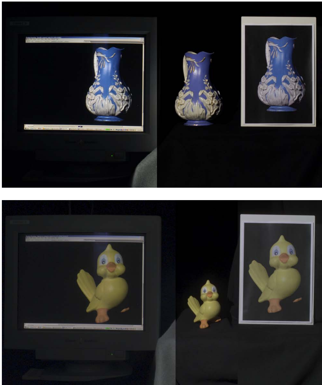
Figure 5.5: Photographic comparison of the appearance model with the original object. The images show a rendered image on a CRT screen (left), the original object under the same pose and illumination conditions (middle), and a color laser printer printout of the rendered model (right). The luminance levels required a longer exposure times for the screen compared to the other parts. The lower image is composed from 3 individual images taken under identical conditions as the model was broken during the acquisition.
