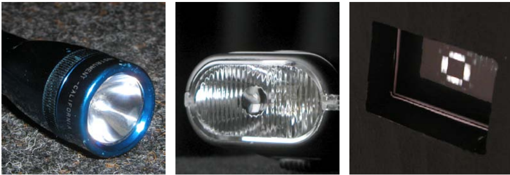
Figure 6.14: Left and middle: Image of the flashlight and the bike light. Right: The negative part of the filter \Phi'_{\text{bellq}} illuminated by the bike light.
