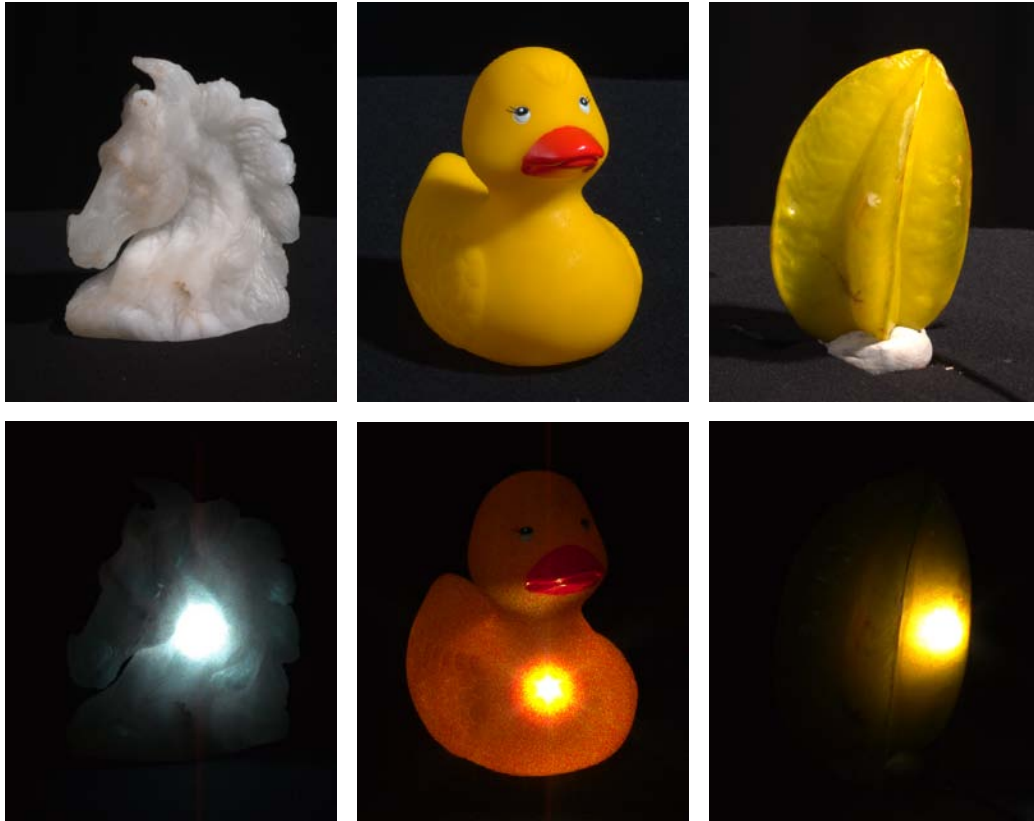
Figure 7.12: Top: The test objects under indoor illumination. Bottom: Test objects illuminated by a white laser beam (all three lasers combined). The laser speckle is strongly visible due to the low fill factor of the camera.
