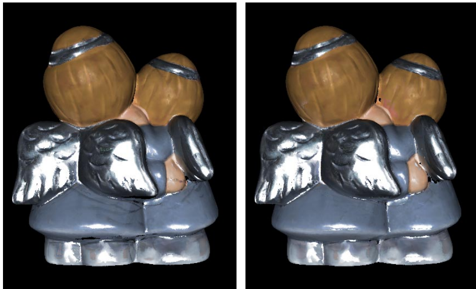
Fig. 5. Left: Dark stripes on the dress and on the hand are due to depth discontinuities. Right: By discarding samples at depth discontinuities and shadow boundaries these effects have been removed.
