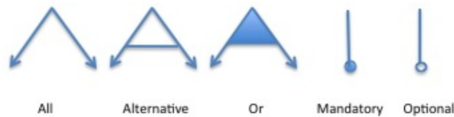
Fig. 4. Feature Diagram Notations: All: all subfeatures must be selected; Alternative: exactly one subfeature must be selected; Or: at least one subfeature must be selected; Mandatory: required feature; Optional: optional feature
