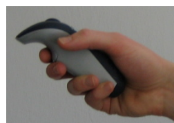
Figure 1. The user holds the gyro mouse in her right hand while conducting.
